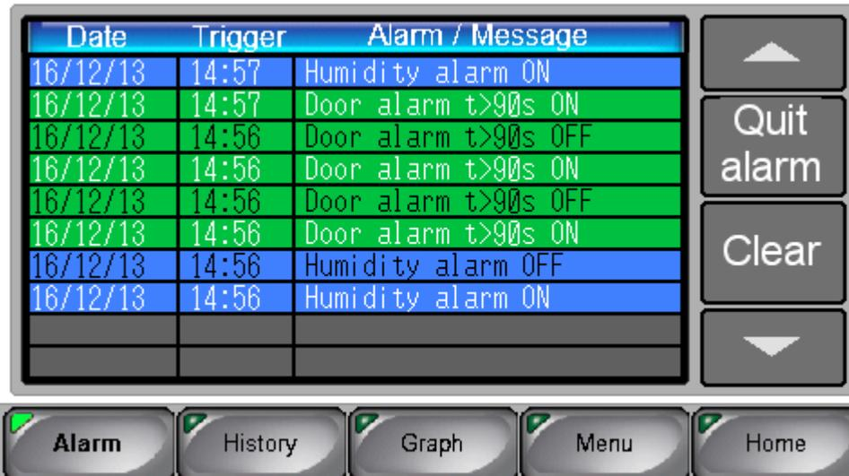
Press [Alarm Acknowledge] to reset the alarm delay. The optical and acoustic alarm signal switches off. If the alarm is still active, the alarm activates again after the set delay time.
